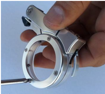
Ref. 1.B Remove 4 cap screws.
