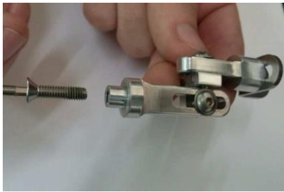
Ref. 1.A Main rod & rod end screw.
